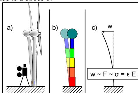
Figure 3: a) Measurement of the displacement of the nacelle by video camera, b) modelling of the tower and c) calculation of the corresponding stresses
