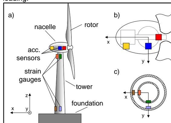
**Figure 2: Measurement system for the assessment of the remaining service life a) as installed on the turbine, b) acceleration sensors in the nacelle, c) strain gauges at the tower base and head**
