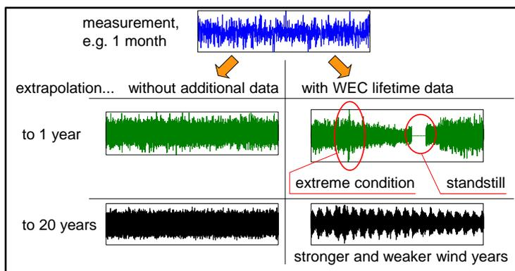
**Figure 1: Extrapolation of short-time measurement data using information about the wind turbine's lifetime (right)**
