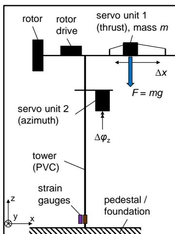
**Figure 4:** Scheme of the test stand: the weight force  $F$  induces a bending moment in the tower base comparable to that induced by thrust on the rotor
